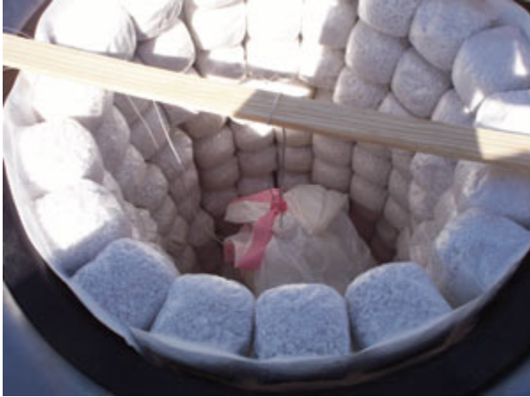
Figure 4: Explosive trial of BlastWrap-lined container. Photo courtesy of BlastGard International
